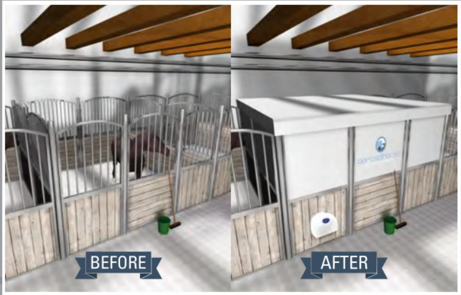
The aerosol is mounted on the outside of the stall. The equipment doesn't occupy much space and it is connected to the inside of the stall through a PVC tube. The aerosol is composed of micronized salt which is then released into the stall (without necessary staff). The aerosol is odorless and very quiet; undisturbed, the animal breathes a flow of "salty" air, where the concentration of salt remain unchanged for the duration of the therapy (usually 30 minutes).
